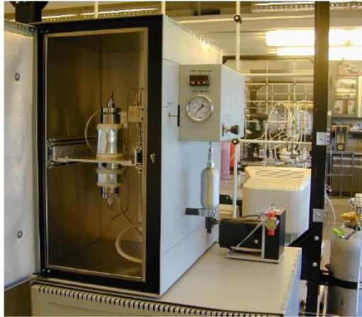
Gambar 27. Supercritical Fluid Extractor (SFE)
