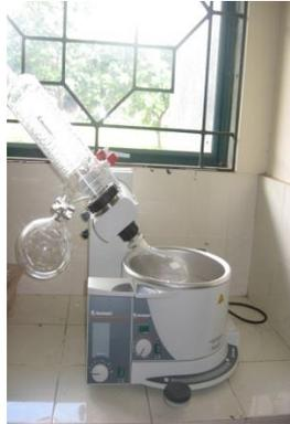
Gambar 15. Evaporator skala laboratorium
