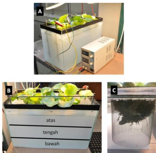
Figure. EAPR system reactor (A) and water sampling point in reactor (B) and pot-shaped cathode (C)
